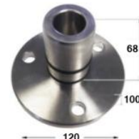
BDH1005x120mm Smaller 68mm Spigot x 120mm Plate - 3 x M13 Fixing Holes 304/316
