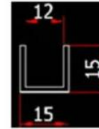
10mm-Shower-Profile 3m Lengths - 10mm Glass Ali - Satin Anodised (Also available in 304G Mirror polish)
